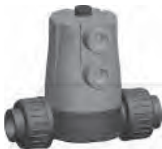
Diaphragm valve type 604 PVC-U Unions with solvent cement socket BS
