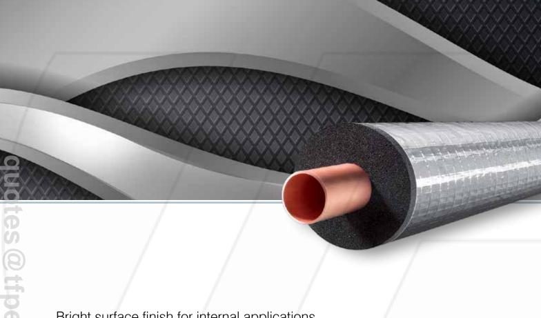
Glass fibre reinforced aluminium foil covering for Kaiflex insulation, Kaiflex Protect Alu-NET protects insulation against mechanical damage and can be supplied either separately as rolls of thin sheet or pre-applied to Kaiflex tube or sheet
