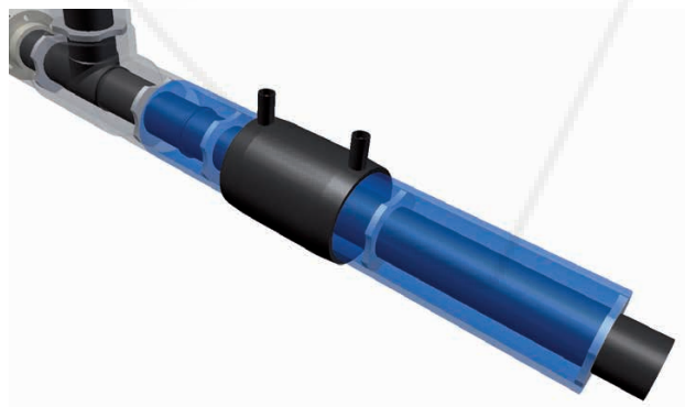
Fig. 2: Alignment of protective pipe for welding
